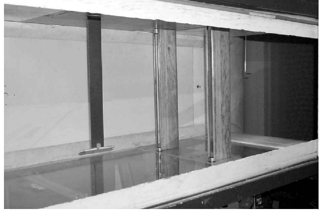
Fig. 2 Experimental model and gust generator in the wind tunnel.
